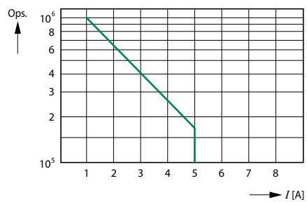
Contact Life (220V 50Hz, AC-1, 360 Operations/hour)
